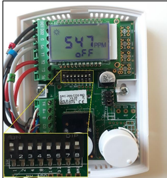
Diagram 5: Location of binary "bit" switches
