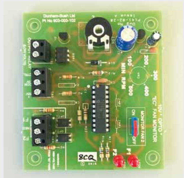
Optional fan monitoring board with relay fault output
