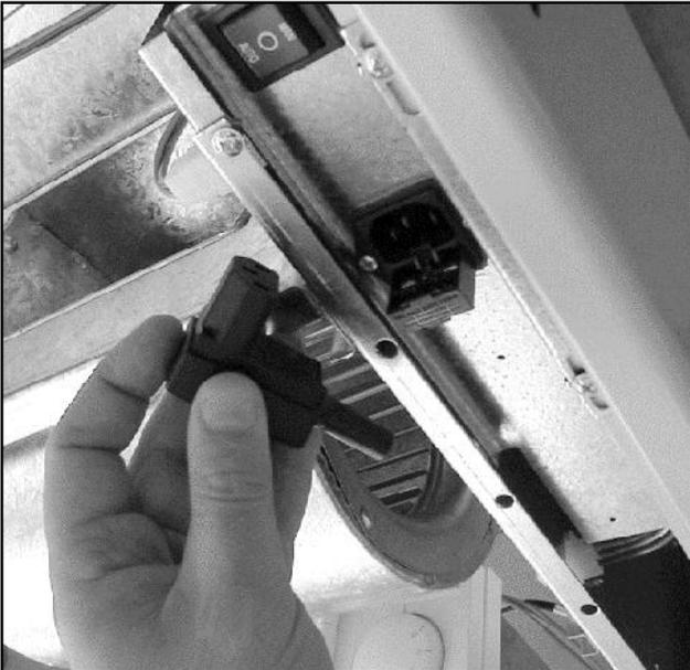
Diagram 3 : Mains inlet plug and fuse holder
