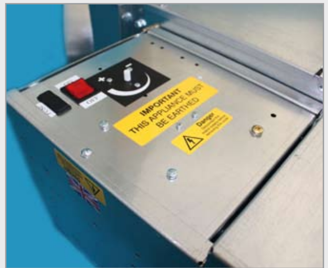
'Panther' control box with fitted speed potentiometer
