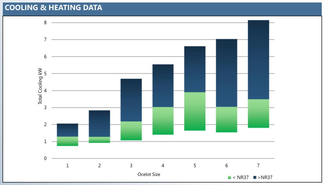
Range of Cooling Outputs - Based on 6/12C CHW and 23C Air On 50% RH. Please contact Dunham-Bush for confirmation of selections.
