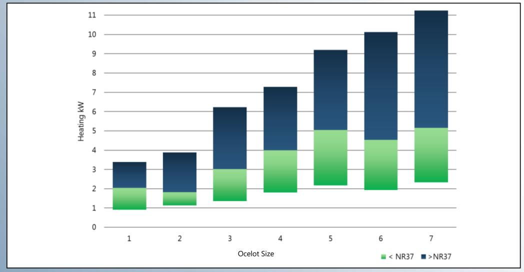
Range of Heating Outputs - Based on 80/70C LPHW and 20C Air On. Please contact Dunham-Bush for confirmation of selections.
